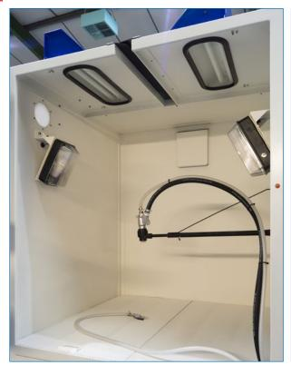
The Guyson Euroblast 9 blast cabinet has been designed to accommodate taller components and is equipped with an upper and lower set of armholes; allowing the operator a choice of blasting positions. Standard Features
